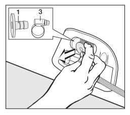
Remove the following from the back of the dryer at the bottom:
